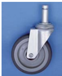
RUBBER SWIVEL 1 1/4" x 5" 200 Lb. Capacity
